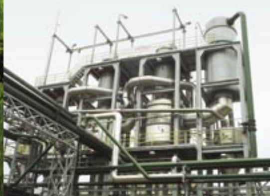
Water produced by the evaporator (above, right) at Unilever's tomato processing plant in Goiânia, near Brasília, Brazil, is recycled for further use in the plant. Globally, Unilever continues to reduce its water use (see graphic above).
